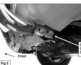
(Fig 4) Driver/left mounting Bracket installation
