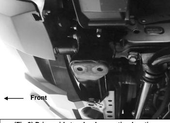
(Fig 2) Driver side tow hook mounting location
