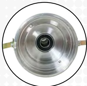
Ball bearing supported shaft
