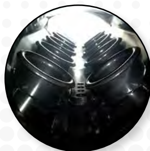
Velocity stacks for better air flow
