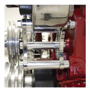
4. Tighten lower bolt on power steering pump. Adjust power steering pump position and tighten upper bolt.
