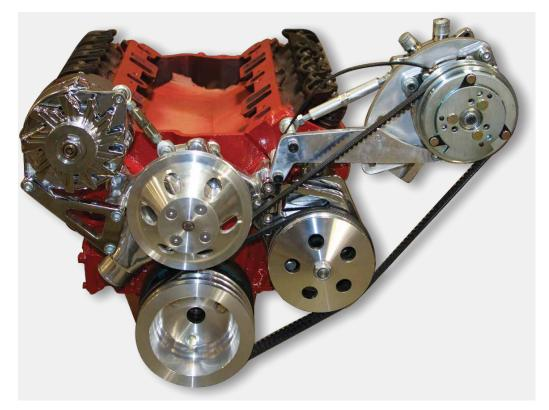
8. Once belt has been placed on the first groove of the A/C compressor , first groove of the power steering pump, and middle groove of the crankshaft pulley, you can adjust the tension of the v-belt by moving the A/C compressor. Once the correct tension is found, tighten bolt that is connected to the compressor bracket and bracket #1 to lock the A/C compressor in to place.
