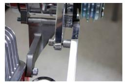
6. Place bolt 1.75 x 3/8-18 with washer threw compressor bracket adjustment slot back. Place 0.556 inch spacer in between compressor bracket and bracket #1. Do not tighten, finger tight.
