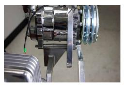
5. Place bracket #2 in between post of A/C compressor. Place 3mm spacer in between front post of compressor and bracket #1. Feed bolt  $5 \times 3/8-18$  with washer threw compressor and brackets. Tighten brackets.
