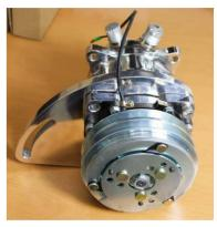
4. Attach compressor bracket with  $1.75 \times 3/8-18$  with washer and nut as shown in figure above. Tighten.
