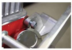
3. Attach bracket #2 with 1 x 3/8 -18 bolt and washer to head. Tighten.
