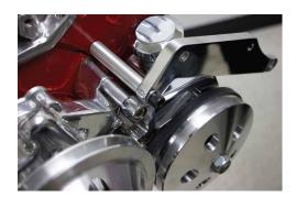
1. Attach bracket #1 with 4.25 x 3/8 -18 hex bolt, 3.25 inch spacer, and washer to bolt. Finger tighten.
