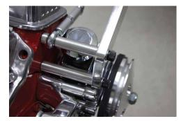
2. Attach bolt 4.25 x 3/8-18 through second bolt opening. Place 2.45 inch spacer against bracket #1. Place adjustable column and 0.30 inch spacer through the bolt. Tighten both bolts.
