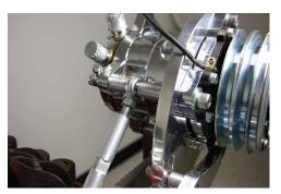
7. Place bolt 5 x 3/8-18 threw un used compressor top mount. Place spacer 1.28 inch first after compressor mount. Attach other end of adjustment column threw bolt and placing 1.0 inch spacer last before. Tighten.
