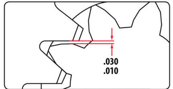
Figure 3 (Ring gear backlash)
