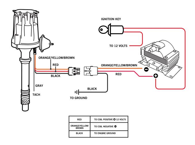
**WARNING:** This distributor is not compatible with stock points distributor coil, must use high output coil. Must bypass ballast resistor if applicable.
