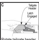
Rotate tailgate header down until both latches engage. Listen for double click.
