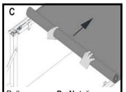
Roll up cover. **Do Not** disengage loop and hook fasteners prior to rolling up cover.
