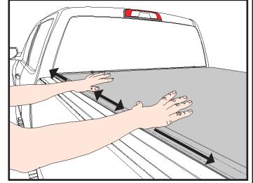
Engaging Hook and Loop, <u>Step Two:</u> With the cover closed and both hook and loop engaged, use the palms of your hand to firmly push the loop strip into the hook track. Do this to both driver and passenger side up and down the entire length of the loop seams.
