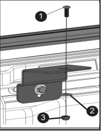
Apply pressure on the rail down and towards the outside of the bed while tightening the bolt to hold rail down to bracket.
