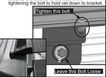
Apply pressure down on the rail and the bracket to compress the rail seal and tighten
