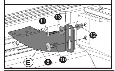
8: Locate the Mounting hole in rail at the front Proceed by lining up that hole with the slot in the front bracket from step 7 and assemble hardware as shown.
