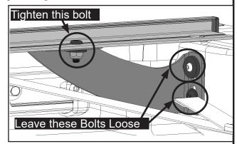
11: Apply pressure on the rail down and towards the outside of the bed while
