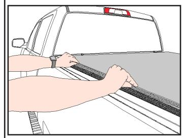
Engaging Hook and Loop, <u>Step One:</u> After rolling the cover closed, grab the fabric loop flap and evenly pull loop over the hook track engaging the loop to the hook track. **Avoid pulling fabric flap straight up.**
