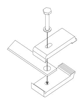
3) With the bolt head facing the logo, place the support bar underneath the rear flap. Close the flap and secure.
