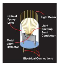
Because filament failure is not a concern for LED lights, they have an extremely fast turn-on time, and can last up to 100,000 hours. Combine this with their durability, and it's clear that they are ideal for the heavy duty industry.
