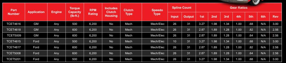
NOTE: Torque and RPM ratings may vary based on vehicle use, drivleline configuration, and quality of product installation.
