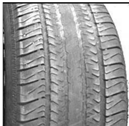
Fast Centerline Wear
