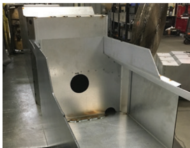
Replacement tanks have internal baffles for extra durability and strength, and to reduce fuel slosh.
