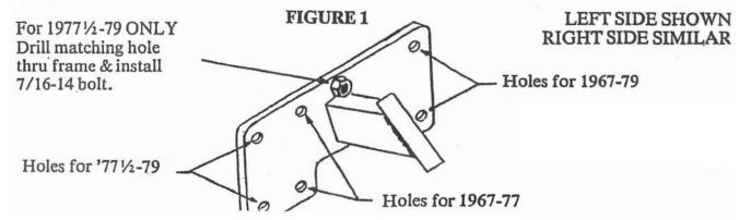
NOTE: ON 1977½-79 MODELS WITH LEAF SPRING FRONT END ONLY, THE HOLES IN THE FRAME DO NOT MATCH THE HOLES IN THE TRANS-DAPT MOTOR MOUNT STANDS. PLEASE FOLLOW THE STEPS BELOW FOR THESE MODELS:
