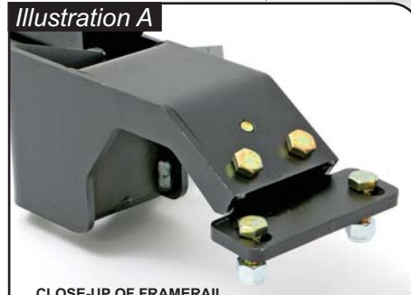
Illustration A CLOSE-UP OF FRAMERAIL CONNECTOR PLATE ASSEMBLY
