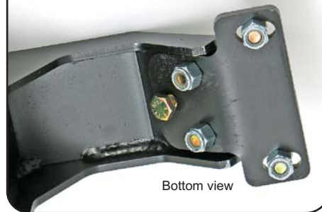
Illustration A CLOSE-UP OF FRAMERAIL CONNECTOR PLATE ASSEMBLY
