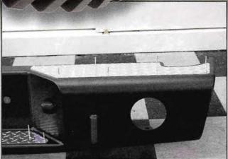
Before securing the top plates to the bumper, I testfit them in place and secured them with the rivets provided in the kit. Then the PIAA 510 Super White driving lights and trailer light mounting plate were installed.
