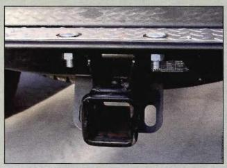
Because TrailReady expects owners to use the functionality of the D-rings on their bumpers, it incorporates extra mounting hardware for the bumper. TrailReady provides two carriage bolts to secure the bumper to the receiver hitch. This makes sure it is securely fastened to the frame and the receiver hitch.
