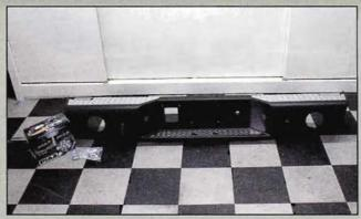
The rear of the truck gets TrailReady's rear bumper, which is constructed pretty much like the front bumper. It also has D-ring mounts for 1-inch shackles. Diamond-extruded aluminum top plates add toughness, while the pair of PIAA 510 Super White driving lights add rear-facing illumination.
