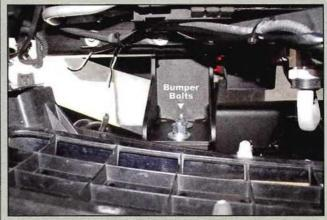
The grille must be in place before the bumper is installed on the truck.
