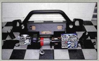
For the front of the truck, we will install TrailReady's extreme-duty front winch bumper made from ¼-inch and  $\aleph_{e}$ -inch steel with quad light ports for 4-, 5-, and 6-inch round lights, and D-ring mounts for 1-inch shackles. A Superwinch EP 16.5 winch, a pair of PIAA 520 ATP Xtreme White lights, and a pair of PIAA 510 Super White driving lights will be installed on the bumper.
