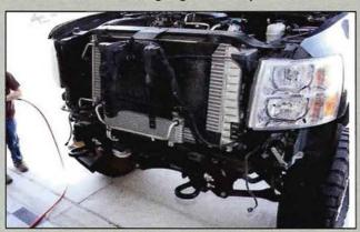
The stock bumper is held in place by six bolts that secure it to the frame. Retain the two dual bolts for use with the new bumper. I disconnected the electrical connector for the foglights and removed the bumper from the truck.
