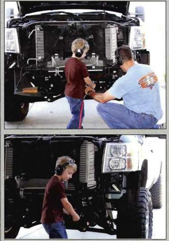
Since TrailReady's bumper comes with D-ring mounts for tow hooks, the stock ones are no longer needed. There are three bolts securing each tow hook to the frame of the truck. Once removed, they easily pull right out.
