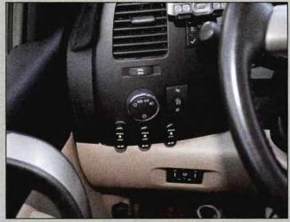
The light switches are routed through the knee panel and secured under the main light switch. Once all the wires were routed and the switches were in place, the installation was complete, but the project wasn't. PIAA offers instruction for the proper control and alignment of the driving lights. There is nothing worse than poorly aligned driving lights. Once the lights were properly adjusted, the project was complete.
