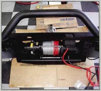
After installing the lights, it was time for the EP 16.5 winch. The bumper is predrilled to accept the 10x4-inch pattern for the roller fairlead. TrailReady's design allows for winches to be mounted footforward or foot down. This is a feature not found in many bumper designs.
