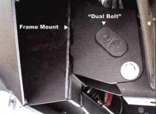
Before the bumper can be installed on the truck, the frame mount is attached to the frame using the OEM dual bolts and hardware provided by TrailReady.
