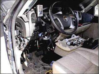
The most time-consuming part of this installation was completing all of the electrical connections. The light kits from PIAA are exceptional. They include everything needed for the installation and the wire harness has multiple connections for ease of installation of the lights, relays, and switch. The control harnesses for the lights are routed into the cab through the firewall and the floorboard.
