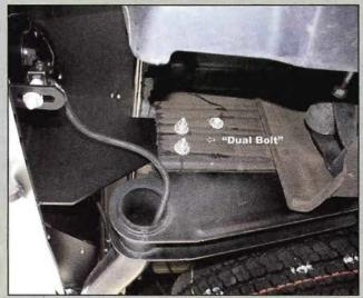
The bumper is secured to the frame using the dual-bolt system and an additional bolt. A replacement nut and bolt is provided for securing the frame to the receiver hitch that was incorporated into the stock bumper.
