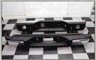
When placed side by side, TrailReady's rear bumper—with its all-steel construction, aluminum diamond-extruded top plate, D-ring, and light ports-makes the DEM look like it should be on a child's toy, not on a heavy-duty truck.
