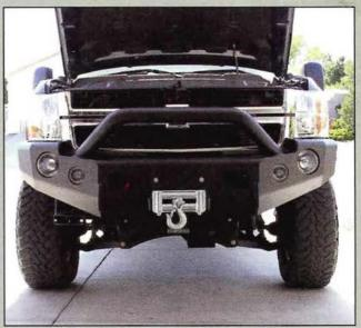
Now it was time to loosely attach the bumper to the frame mounts. TrailReady's mounting system allows for adequate horizontal and vertical adjustment of the bumper for a perfect alignment. The bumper is secured to the frame mount using 8½x1½-inch Grade 8 carriage bolts.
