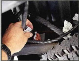
First, I removed the electrical connector for the license plate lights and trailer lights. Then I removed the dual bolt system, which attaches the bumper to the frame and the bolt through the receiver hitch. Repeat for the other side.
