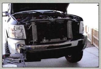
The first order of business was to remove the plastic top cover and grille to gain access to the bolts securing the bumper to the frame. There are eight plastic rivets, which attach the grille to the plastic cover, and six pinch clips. There are also four 10mm head bolts securing the grille to the body of the truck.
