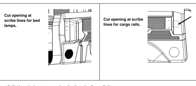
Drill 19mm holes at center of scribe lines for Cargo Rails.
