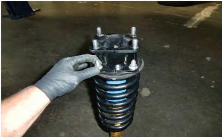
Install the strut extension to the strut using the factory hardware. Install the completed strut into the frame using the provided hardware. Raise the lower control arm to the strut and install the factory hardware. Install the lower ball joint cradle to the knuckle using the factory hardware.
