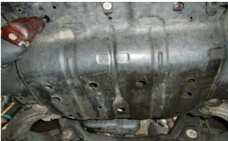
4WD steps: Remove the factory skid plate.
