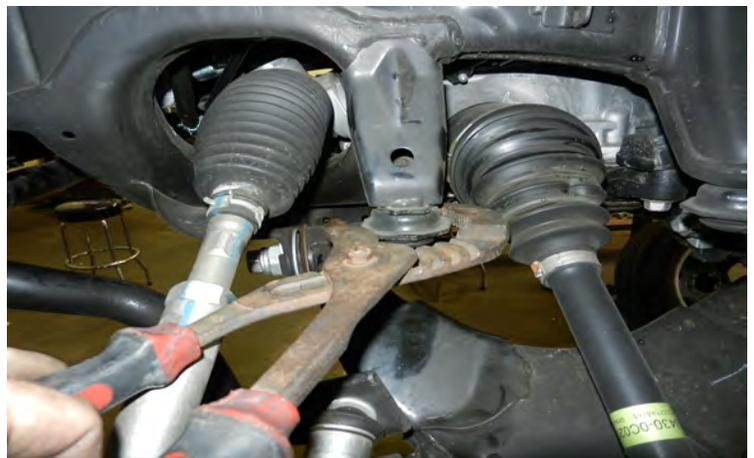
Remove the lower control arm bump stops.
