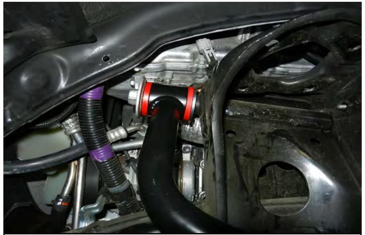
Install the upper control arm making sure to install the provided washers on the inside mounts. Reuse the factory washers on the outside of the arm.
