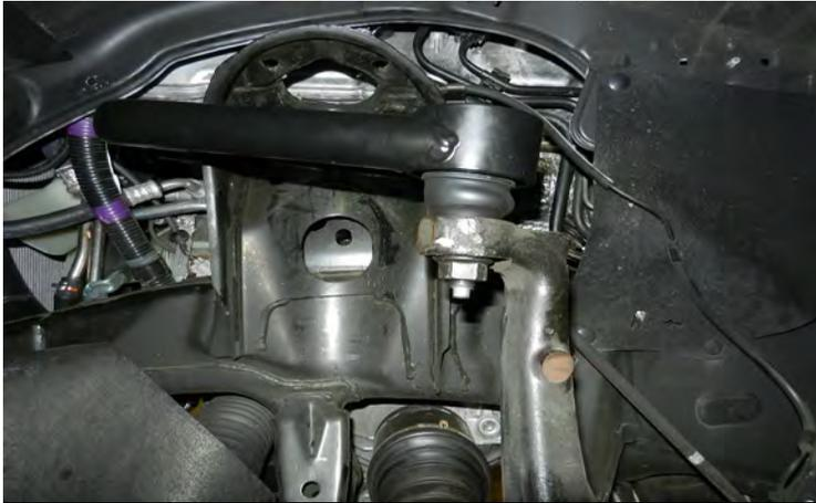
Install the knuckle to the upper ball joint using the provided hardware.
