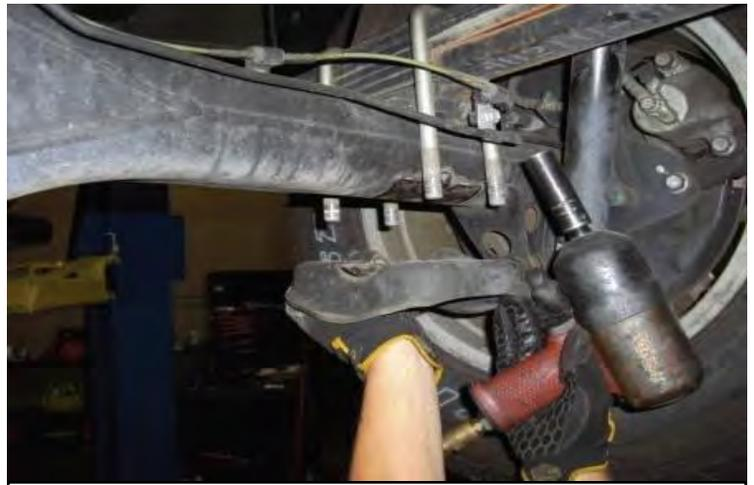
Remove the u bolts on the side you intend to work on first. Lower the axle low enough to insert the provided lift blocks. Install the provided u-bolts and axle cradle. Repeat for the other side of the vehicle.
