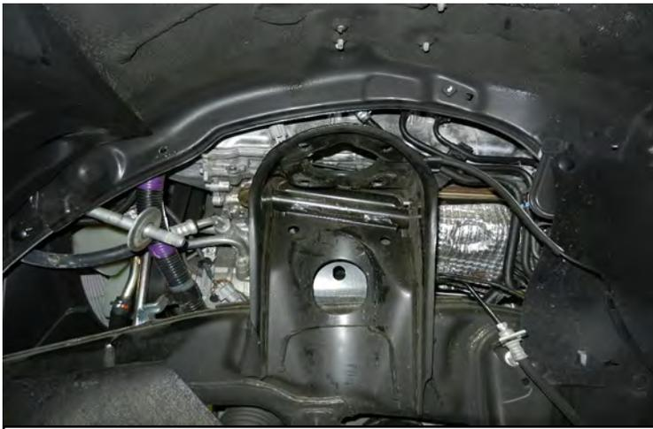
Remove the upper control arm from the frame. (Strut shown removed for clarification. Will be removed in a later step.)
