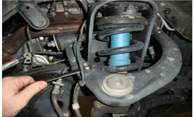
Remove the brake line bracket from the upper control arm. Remove the brake caliper and hang out of the way. Remove the brake rotor.
