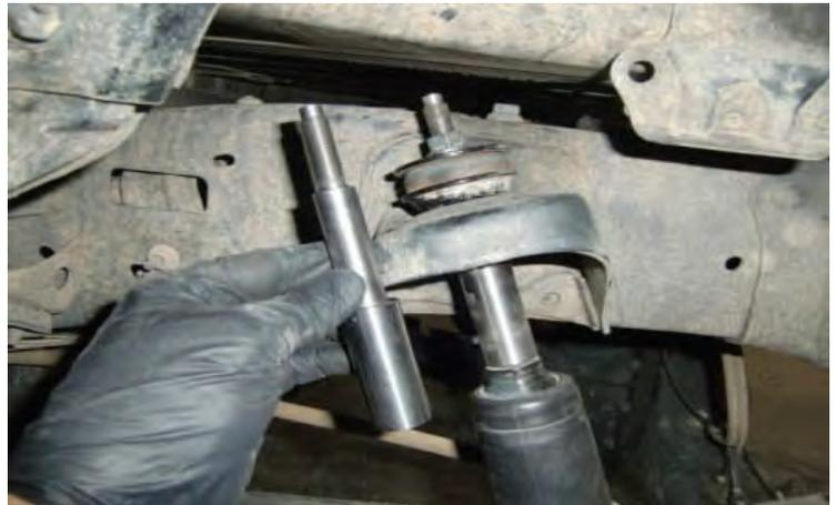
Install the provided shock extensions to the shock. Install the shock back to the vehicle using the factory hardware. Install the brake line brackets back to the axle. Make sure everything is torqued down and there is clearance for the tires against all moving parts. Have the alignment set.
