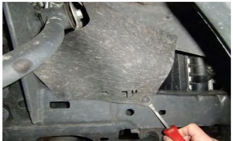
Remove the front splash guards from the frame for access to the upper control arm bolt.
