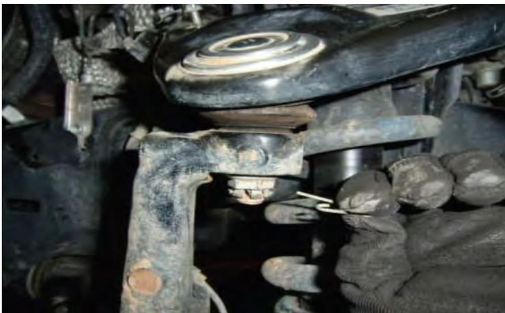
Remove the upper ball joint safety clip and nut. Strike the ball joint boss with a dead blow hammer to dislodge the taper.
