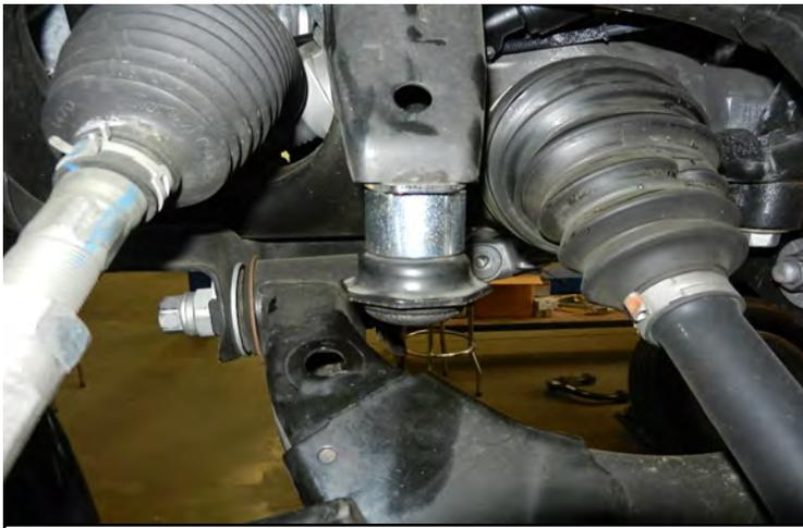
Install the provided bump stop extensions to the frame and the bump stops to the extensions.
