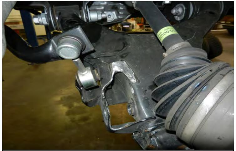
Notch the lower control arm strut pocket as shown using a suitable cutting device. Sand any burrs off the cut edge. Paint the cut area with a quality rust preventative paint.
