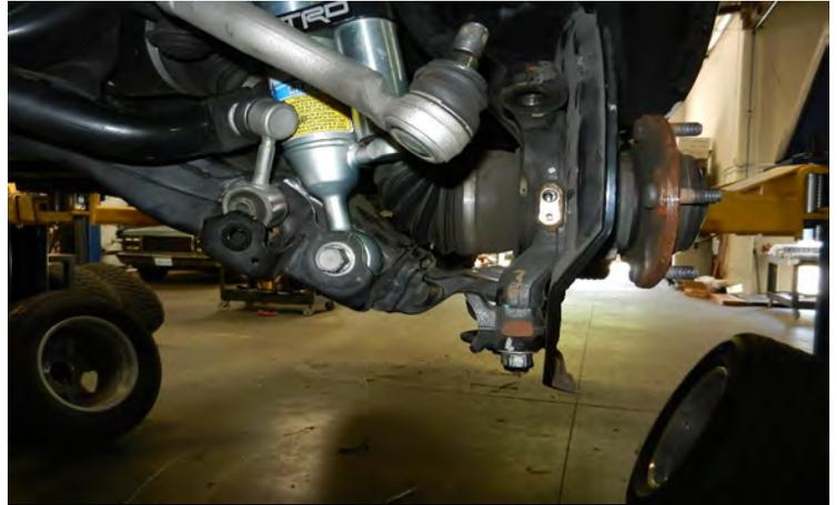
Remove the sway bar from the lower control arm. Loosen the lower control arm bolts.
