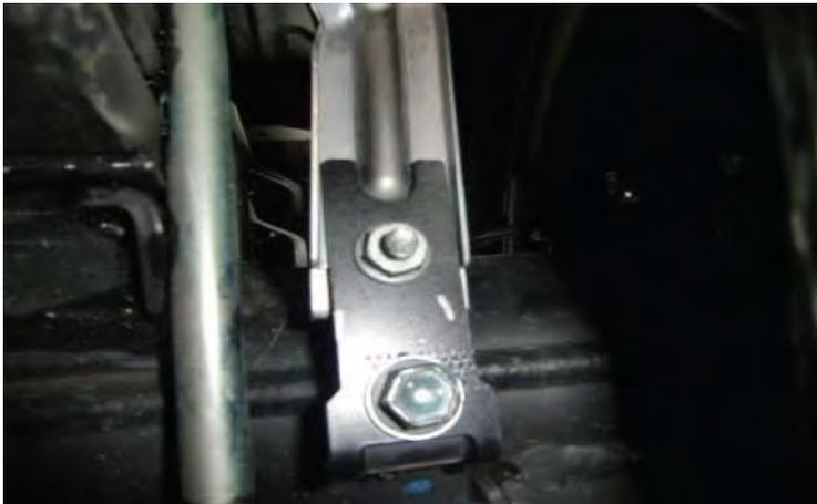
Install the parking brake cable brackets to the axle and the factory mounts using the provided and factory hardware.
