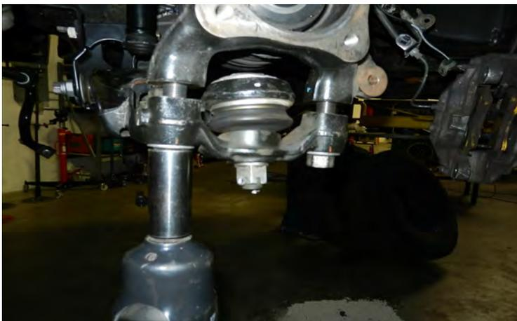
Remove the lower strut bolt. Remove the ball joint cradle bolts and let lower control arm swing out of the way. Remove the strut from the vehicle.
