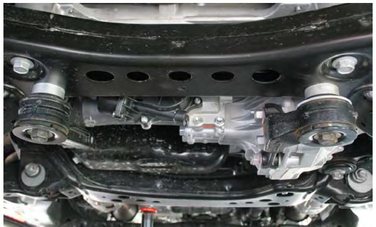
Remove the front diff mount to frame bolts. Lower the diff low enough to insert the provided diff spacers. Install using the provided longer hardware.
