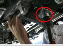
2. Remove the factory 19mm differential mounting nuts and bolts. The OEM washers will be reused.
