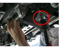
1. Position a floor jack under the front differential. Raise the pad so that it is touching the diff.
