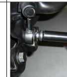
Using a 19mm socket, loosen and remove the sway bar end link bolt on the lower control arm.
