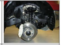
Starting on the driver side, remove the five lug nuts and the wheel.
