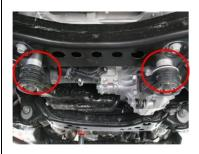
3. Install the 1" spacers between the differential supports and the front crossmember. Install the new bolts with factory washers and the new nuts and washers. Torque to factory specs.
