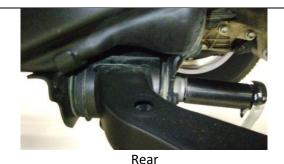
Using a 24mm socket, loosen but don't remove the driver side lower control arm bolts. This will allow the lower control arm to move freely.
