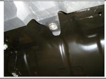
Remove the skid plate. Some models may have two skid plates. A 12mm socket is needed.
