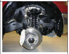
Install the two 22mm lower ball joint bolts starting with the rear bolt first, as it is easier to line up with the spindle. Torque to factory specs, use thread locker where necessary. Tighten the four 14mm upper strut mounting bolts and torque to factory specs. Put the wheel back on and torque to 85-90 ft/lbs. With vehicle on the ground tighten the lower control arm bolts and torque to factory specs. Use thread locker where necessary.
