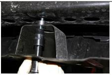
Using the hardware provided, install the M8 bolt, washer, skid plate, and 1/2 tall spacer into the back two skid plate mounting points. Use the OEM hardware for the two front mounting parts.
