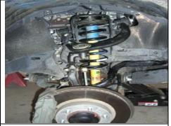
6. Reinstall the strut assembly in its stock location. Leave the three upper strut mounting nuts loose Raise the lower control arm and install the lower strut mounting bolt and nut. Use a floor jack to raise the lower control arm up in order to get the lower ball joint bolts installed. Be sure to use a thread locker on the lower ball joint bolts.
