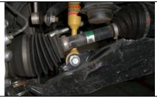
2. Starting from the passenger side, loosen the up-per and lower strut mount nuts.
