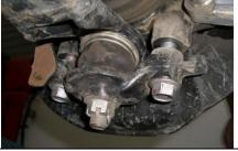
**3**. Loosen, but do not remove the 19mm lower con-trol arm nut and bolt, Remove the 19mm lower ball joint bolts.
