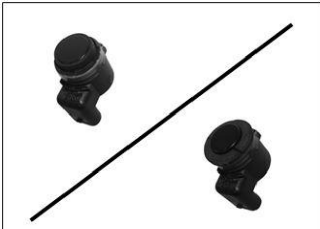
(Fig 10) Remove OE sensor washer and place the provided Foam Washer onto the front of the sensor
