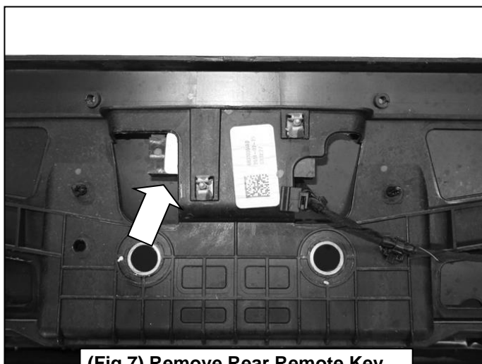
(Fig 7) Remove Rear Remote Key Antenna from behind bumper
