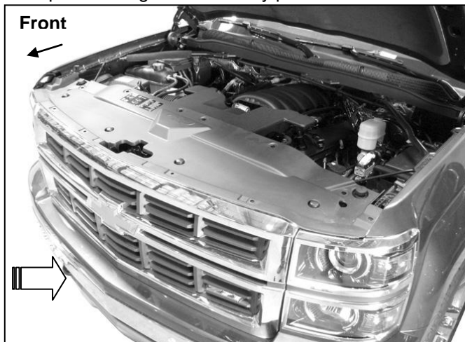
(Fig 2) From behind bumper, release clips along the center and the hardware at the fenders attaching the plastic facia panel (arrow) to top of bumper. Remove facia panel to access bumper hardware
