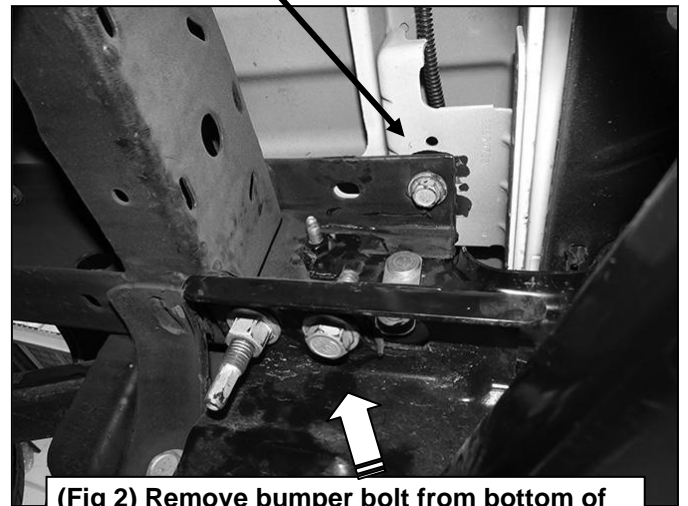
(Fig 2) Remove bumper bolt from bottom of frame (arrow). Back of passenger side of model w-o receiver hitch pictured from below
