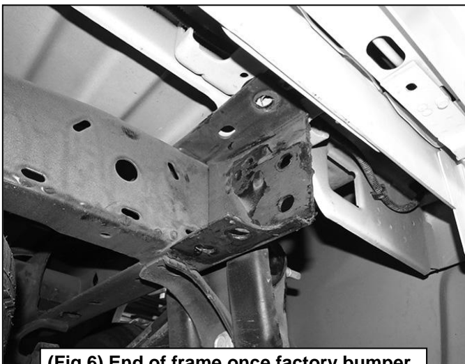
(Fig 6) End of frame once factory bumper is removed. Passenger side w-o receiver hitch pictured
