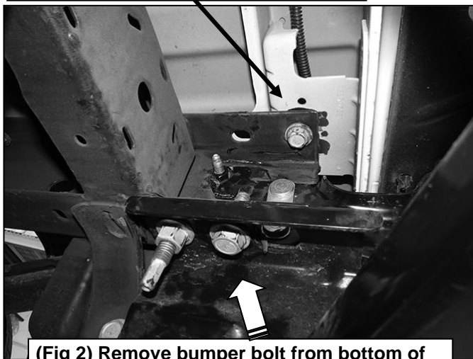
(Fig 2) Remove bumper bolt from bottom of frame (arrow). Back of passenger side of model w/o receiver hitch pictured from below
