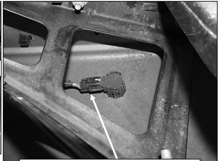
(Fig 2) Unplug the sensor first then remove the sensor from the mounting sleeve
