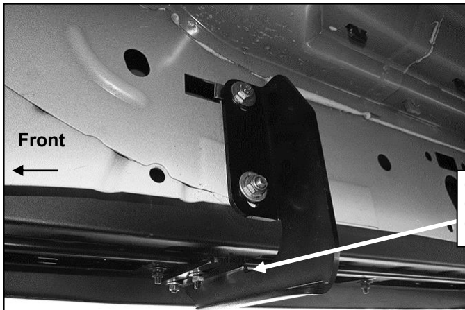
(Fig 10) Passenger/right front Bracket installed
