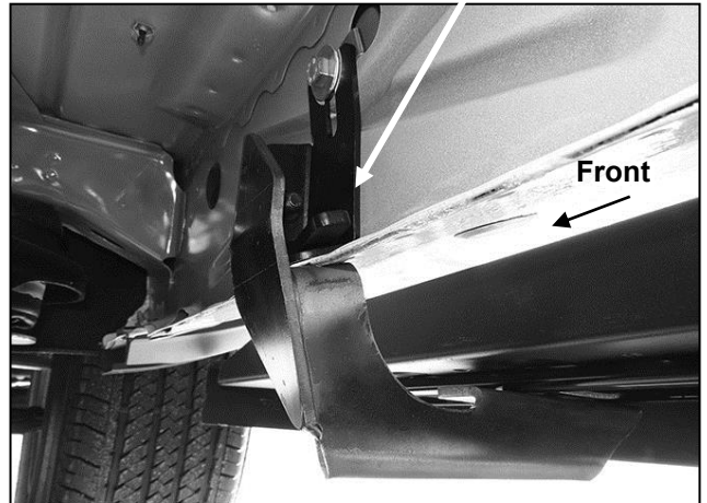
(Fig 17) Passenger/right front Bracket installation
