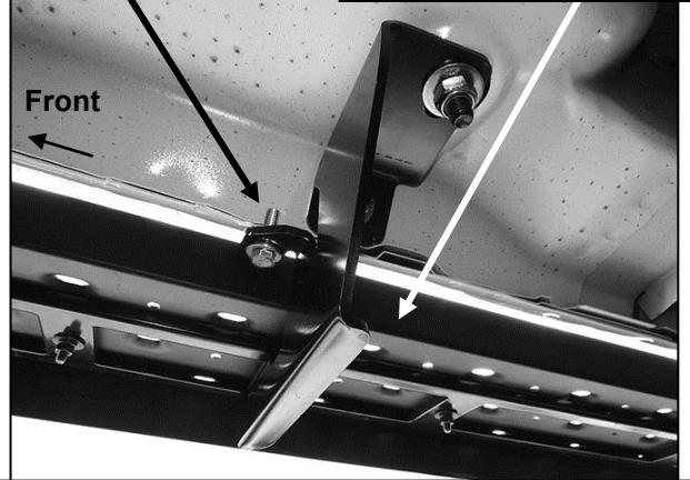
(Fig 24) Passenger/right #2 Bracket installation
