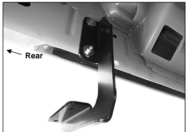
(Fig 7) Driver/left rear Mounting Bracket installed
