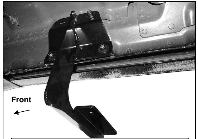
(Fig 5) Passenger/right front Bracket installed
