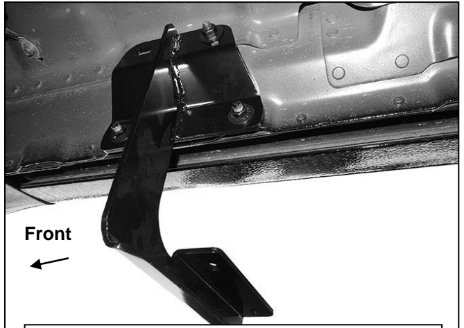
(Fig 5) Passenger/right front Bracket installed
