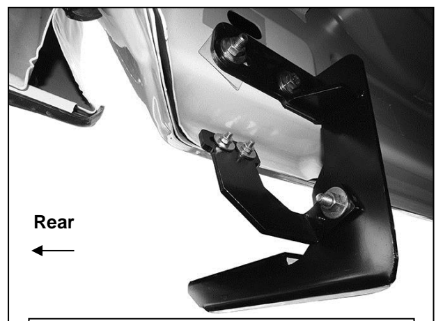
(Fig 17) Driver/Left rear Brackets installed
