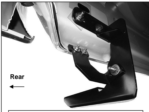
(Fig 17) Driver/Left rear Brackets installed
