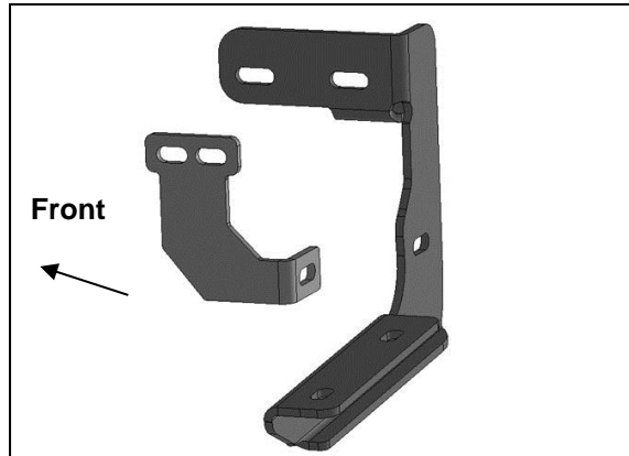
(Fig 6) Driver side front and center Brackets
