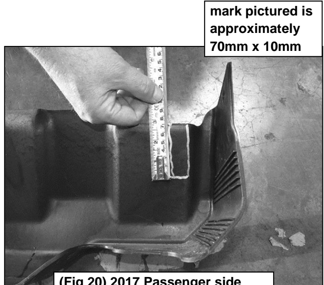
(Fig 20) 2017 Passenger side DEF cover marked for trimming
