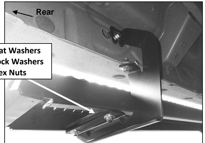
(Fig 11) Driver/left rear Bracket installed
