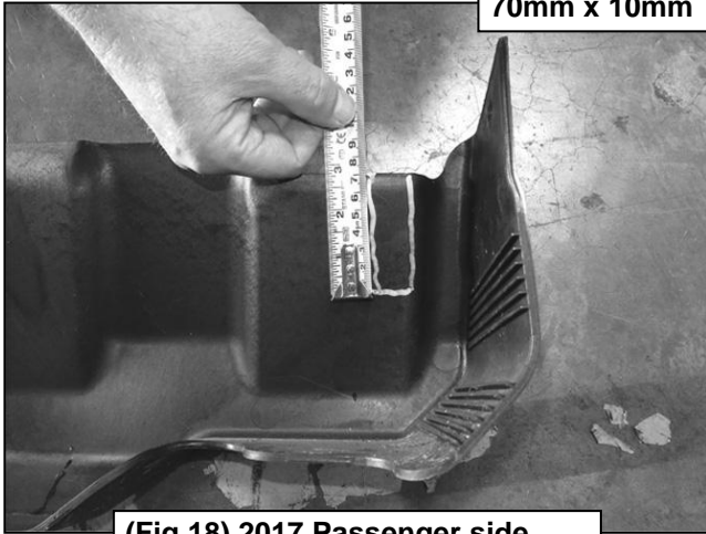
(Fig 18) 2017 Passenger side DEF cover marked for trimming
