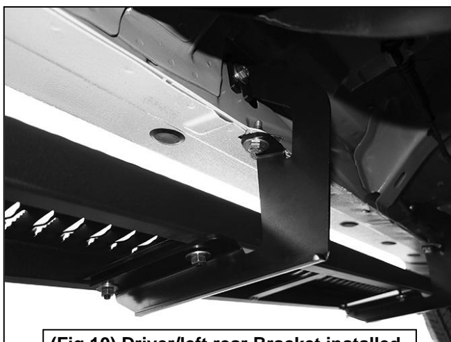
(Fig 10) Driver/left rear Bracket installed
