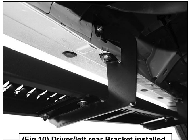
(Fig 10) Driver/left rear Bracket installed
