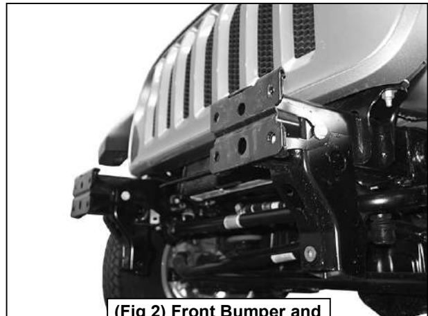
(Fig 2) Front Bumper and splash guard removed
