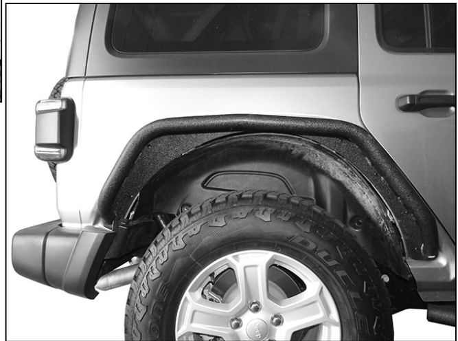
(Fig 13) Attach rear of Fender to mounting locations on body, (pass/right Fender pictured)
