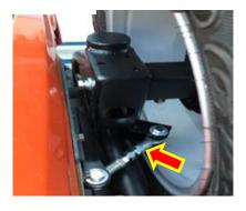
M12x70x2 bolts M12x30x2x4 Flat Washers M12 x2 Spring Washers one set of Tie Rod Assembly four Tie Rod Gaskets
