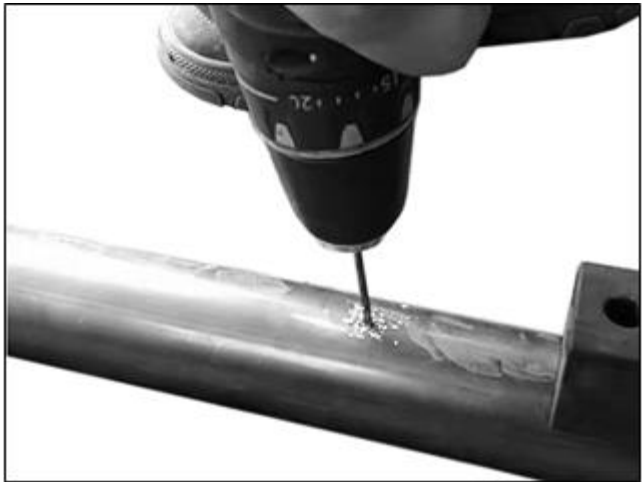
(Fig 22) Drill 1/8" pilot hole
