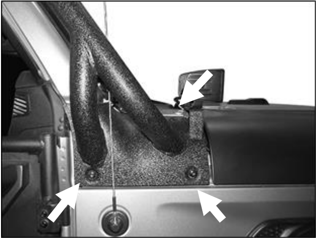
(Fig 7) Reuse factory bolts to attach passenger/right Front Rack Leg to body (arrows). Accessory light not included
