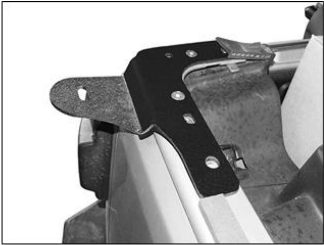
(Fig 12) Passenger/right Mounting Bracket installed
