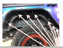
Install bolts and nuts on the corresponding hole.
