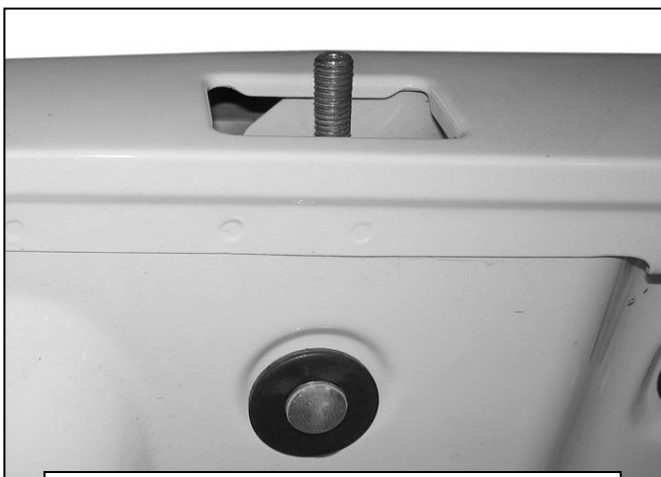
(Fig 5) Use the 10mm J-Bolt to secure the front mounting holes on the Bracket to the stake pocket if possible. Do not drill any mounting holes until after all mounting locations are checked for clearance
