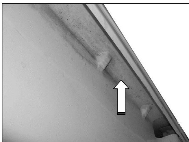
(Fig 6) Before drilling any holes through the top of the bed, check the bottom of the top edge of the bed for hardware clearance.
