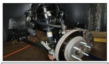
Park vehicle on a clean flat surface and block the rear wheels for safety. Engage the parking brake. Disconnect the vehicle power source at the ground terminal on the battery. Raise the front of the vehicle and support with jack stands at each frame rail behind the lower control arms. Remove the front wheels
