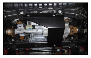
Install the ReadyLIFT® skid plate to the frame cross members using the provided self tapping bolts. Do not over tighten to keep from stripping out the holes in the frame.
