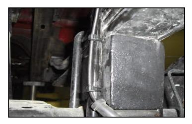
Run the ABS line up next to the block, zip tie to the u-bolts to use as a guide. Reinstall the ABS clip back to the frame. You may need to lube the ABS rubber sleeve to slide it further up to line and back into the clip.
