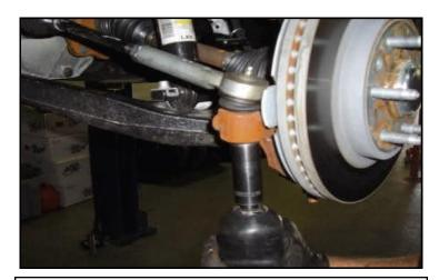
Remove the outer tie rod. Strike the tie rod boss with a dead blow hammer to dislodge the taper.
