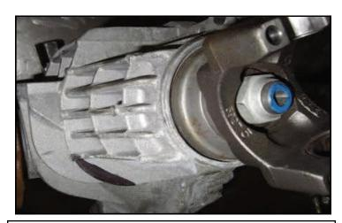
Mark the lowest cooling fin as shown, use a suitable cutting tool, remove the fin. This is for clearance against the driver side rear control arm pocket.
