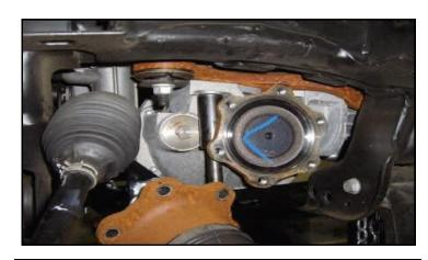
Fully support the differential with a suitable jack. Remove the driver side differential from the hanger.
