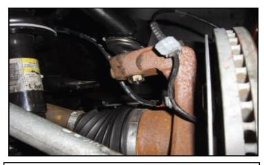
Attach the upper ball joint to the knuckle using provided hardware. Torque to 85 ft-lbs.
