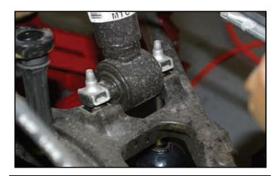
Remove the lower strut hardware from the lower control arm
