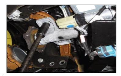
Remove the passenger side differential from the hanger.
