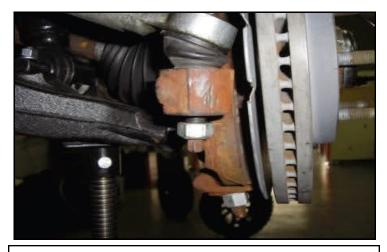
Install the outer tie rod to the knuckle using factory hardware. Torque to 65 ft-lbs.
