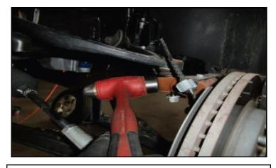
Loosen but do not remove the upper ball joint nut. Strike the ball joint boss with a dead blow hammer to dislodge the taper. Let knuckle hang out of the way making sure to not let the brake line over extend.
