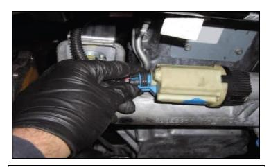
Disconnect the differential solenoid plug and differential vent tube.
