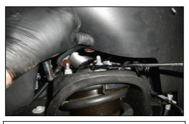
Remove the harness clips from the top of the strut studs. Remove the upper strut mount from the frame. Remove strut assembly from the vehicle.
