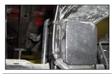
Run the ABS line up next to the block, zip tie to the u-bolts to use as a guide. Reinstall the ABS clip back to the frame. You may need to lube the ABS rubber sleeve to slide it further up to line and back into the clip.
