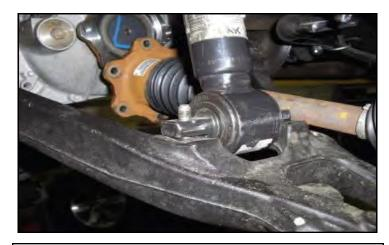
Remove the lower nut clips from the strut. Install the completed strut assembly into the vehicle using M10 flange nuts at the frame and M10 X 60mm bolts, washers, and nuts for the lower control arm. Do not tighten at this time.
