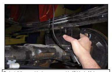
To install the new block passenger side lift block. Make sure the small end of the block is facing the front of the vehicle. Raise the axle and the block up to the spring while aligning the center pin. Install the provided u-bolts, and nuts. Snug the u-bolt nuts but do not fully tighten at this time. Repeat steps for driver side.
