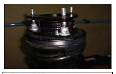
Install the ReadyLIFT® strut extension to the factory strut using factory hardware. Torque to 25 ft-lbs.
