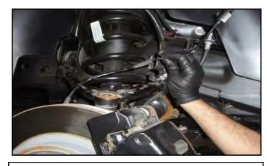
Support the lower control arm with a suitable jack. Loosen but do not remove the lower control arm bolts. Disconnect the ABS connector at the frame. Remove the brake line bracket on the upper control arm.
