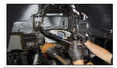
Remove the upper control arm cam bolts. Note their orientation and locations. They will need to be reinstalled the same way as removed. Remove the upper control arms from the frame.
