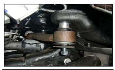
Remove the bolts holding the hangers to the frame. Lower the differential down until you can insert the provided diff drops into place. The large spacers go in between the front side of the hanger and frame and the small spacers go in between the rear side of the hanger and frame. Install using
