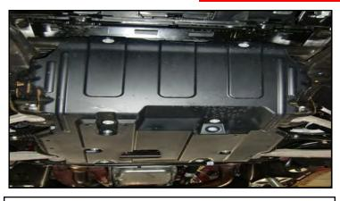
Remove the plastic gravel guard and support the front differential with a suitable jack.
