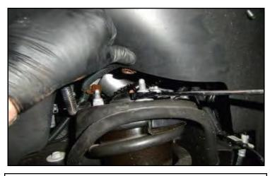
Remove the harness clips from the top of the strut studs. Remove the upper strut mount from the frame. Remove strut assembly from the vehicle.
