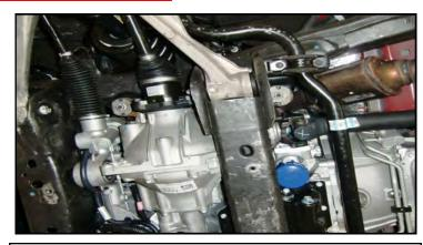
Locate the 4 mounting points of the differential hangers to the frame. These points will not be mounted to the differential directly, but to the hangers that hold the differential.
