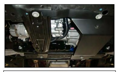
Install the provided skid plate to the frame using factory hardware. Swap the metal bracket from the passenger side of the gravel guard back to the frame. Discard the driver side. Torque to 5 ft-lbs. Make sure to not over tighten and strip out the frame holes. These are self tapping bolts.
