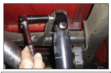
Install the provided shock extension to the frame using factory hardware. Install the factory shock to the extension using M14 x 75mm bolts, washers, and nuts. Install the lower shock to the axle using factory hardware. Do not tighten at this time.
