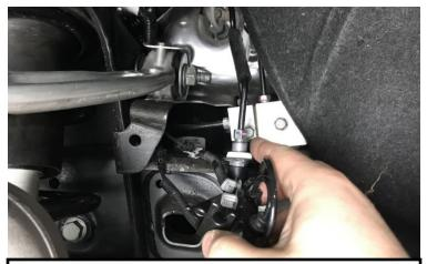
Remove ABS Bracket from UCA; Remove the brake line bracket from Knuckle.
