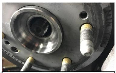
Remove Axle nut and press axle back through hub to allow the knuckle to swing out of the way.
