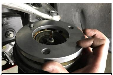
Lower the strut out of the frame. Install the tapered shim onto the strut with the thick end facing outwards. Install the upper strut using the factory hardware. Only install the back nut for now. Do not tighten all the way.
