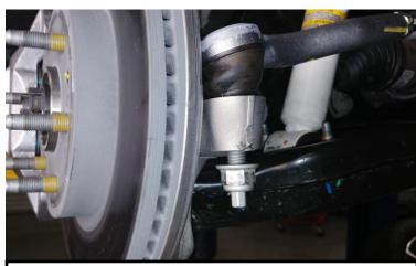
Loosen the tie rod end nut. Strike the tie rod stud with a hammer to dislodge the taper. Remove tie rod from knuckle.
