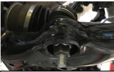
Support the lower control arm with a suitable jack. Remove the front wheels. Remove the sway bar from lower control arm and let hang.
