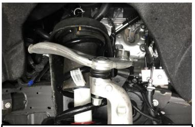
Loosen the upper ball joint nut. Strike the upper ball joint boss with a hammer to dislodge the taper. Remove Ball joint from knuckle. Remove the upper and lower strut hardware. Lower the control arm to gain clearance to remove strut.
