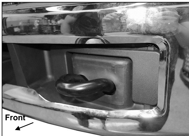
(Fig 5) Remove plastic cover around tow hook
