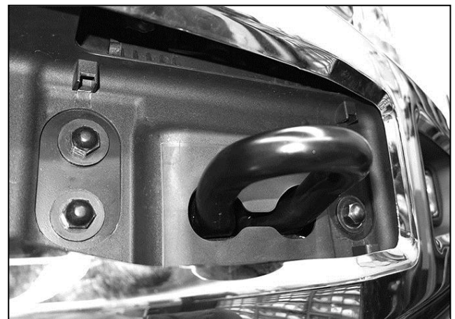
(Fig 6) Remove bumper bolts (driver side pictured)
