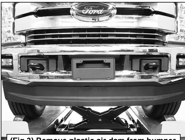
(Fig 3) Remove plastic air dam from bumper
