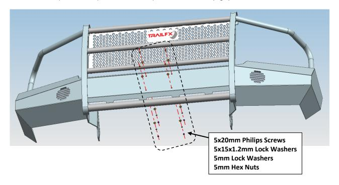
3. Install replacement front bumper on the frame with the hardware, then install the OEM tow hooks (Fig 4A & 4B).
