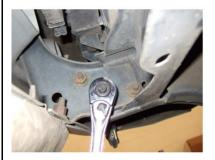
5. With Bumper Supported remove the fasteners and remove by pulling down and out away from the truck.
