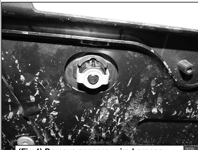
(Fig 4) Remove sensors, wire harness, license plate lights, trailer plug and spare tire access lock (pictured) if equipped
