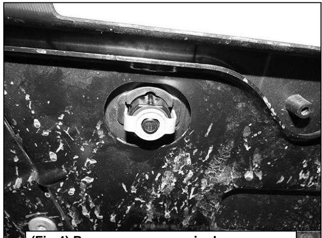
(Fig 4) Remove sensors, wire harness, license plate lights, trailer plug and spare tire access lock (pictured) if equipped
