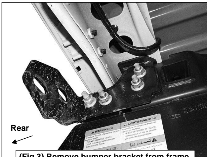
(Fig 3) Remove bumper bracket from frame
