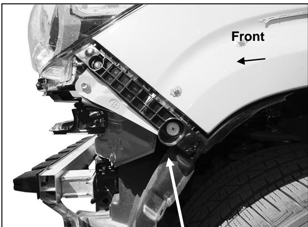
(Fig 3) Remove plastic block from front edge of fender. Reinstall hardware to secure headlight
