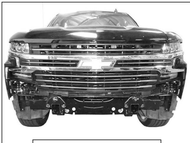
(Fig 7) Reinstall grille and cover
